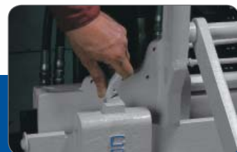
Platens are hung like conventional forks so spacing can be adjusted in seconds (carriage mount models).
